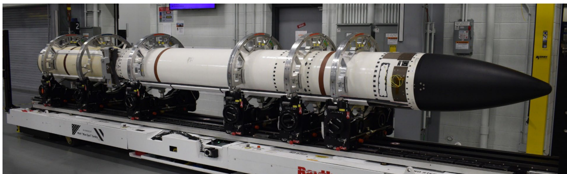
SM-3 Block IIA in final assembly at Raytheon Redstone Missile Integration Facility, located in Huntsville, Alabama.
