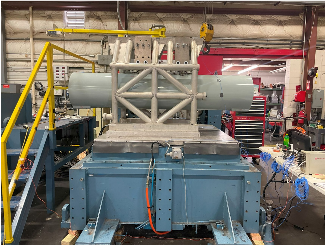
Figure 4 The KIHOMAC team performed a full suite of qualification testing – including 3-axis vibration – on the Advanced Travel Pod
